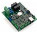
Door Controller RS485
