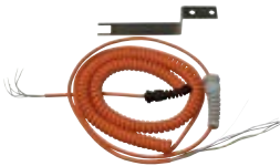
CA0455A00 Spiral cable 5 x 0,5 qmm, 0,8 m spiraled / 3 m stretched.
